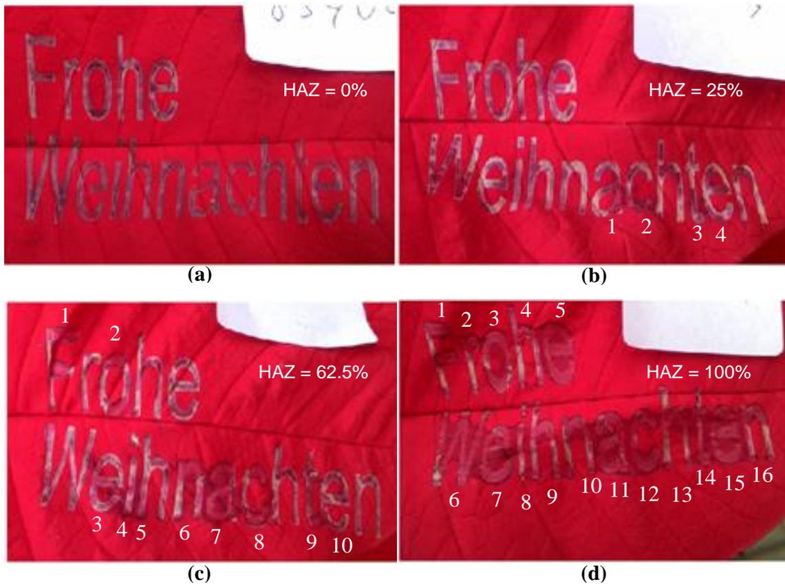
Fig. 5.19. Different levels of heat affected zones (HAZ) 3 days after laser marking on poinsettia leaf, with white numbers showing the calculation of damages on each character; (a) No apparent HAZ; (b) Slight HAZ; (c) Moderate HAZ; (d) Severe HAZ
